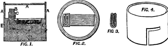
AA is the tinplate cover; EE the gas pipe forming the body of the lamp; BB is the wick which is best if of the "Freiberg" kind, broad, thin, and folded; C is the wick-holder of tinplate, soldered on to E; D is the wax or composition.
