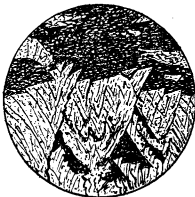
Fig. 3. Vertical section of part of the same specimen as that used in fig. 2, showing cones developing in the argillaceous matrix, which has only in part been forced to assume a definite arrangement. \times 18 .
