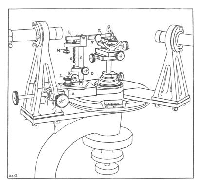
arm E, and carries at its end a socket to receive the shank of the screen G. The spring rests against the point of the fine screw N, which passes through the slightly bent end of E.
