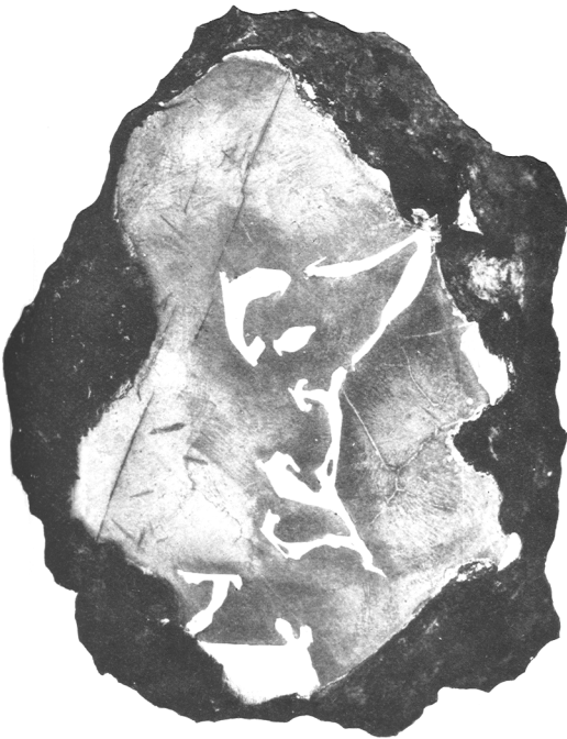
Fig. 2.—Etched surface of the Angela Meteoric Iron showing Schreibersite. (Natural size.)
