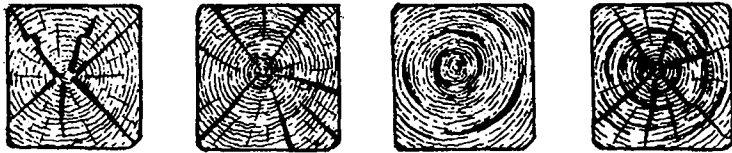
FIG. 1.—Cracks in timber.
