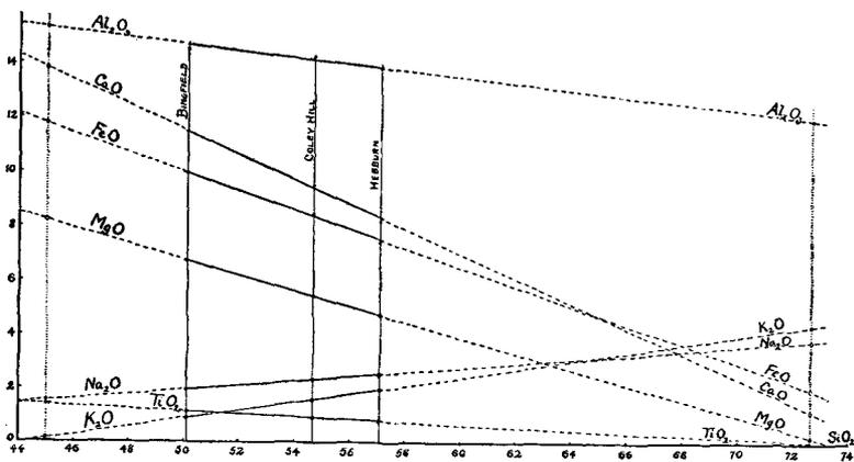
FIG. 4. Linear variation-diagram of the Bingfield-Coley Hill-Hebburn dike-system.
