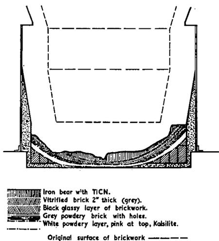
FIG. 2. Section of hearth of blast furnace, showing zoning of deposits.
