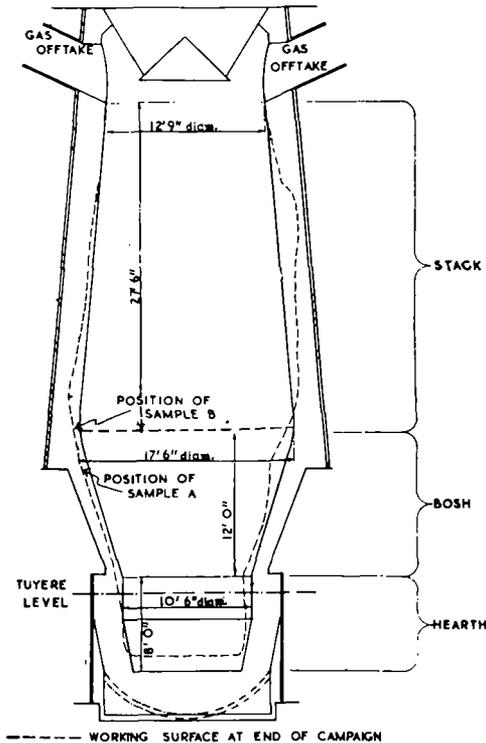
FIG. 1. Section of Kettering no. 3 blast furnace, showing extent of wear of firebrick lining and position of specimens A and B.
