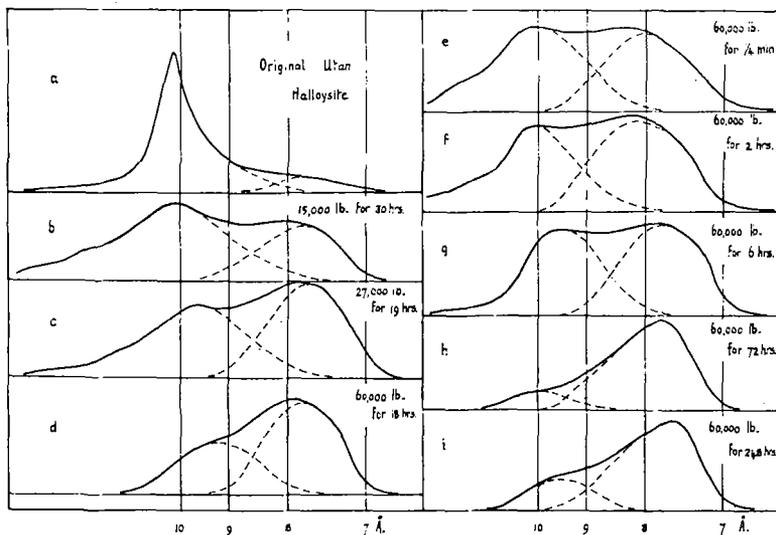
FIG. 3. Microphotometer traces of the (001) X-ray reflection from Utah halloysite before and after application of pressure. A load of 60,000 lb. corresponds to a pressure of 76,000 lb./sq. in. or 27,200 kg./sq. cm. Vertical lines indicate positions corresponding to lattice spacings of 10, 9, 8, and 7 Å.
