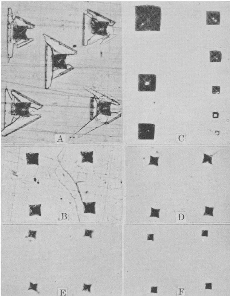
FIG. 1. Hardness of minerals shown by indentations with a diamond point.
