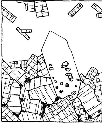
FIG. 3. Halite-anhydrite-magnesite-rock, showing replacement of anhydrite by a large crystal of quartz. 3838-40 feet. \times 32 .
