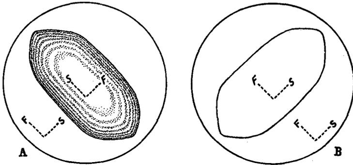
FIG. 1. Zircon between crossed nicols, using high-order plate.
