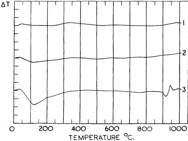
FIG. 3. Thermograms for muscovite: 1. Filed; 2. Ground for 2 hours; 3. Ground for 24 hours.
