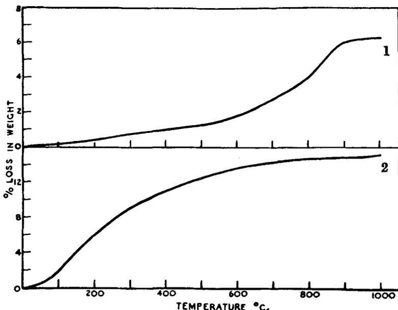
FIG. 4. Dehydration curves for muscovite: 1. Filed (Ca-saturated); 2. Ground for 24 hours (Ca-saturated).
