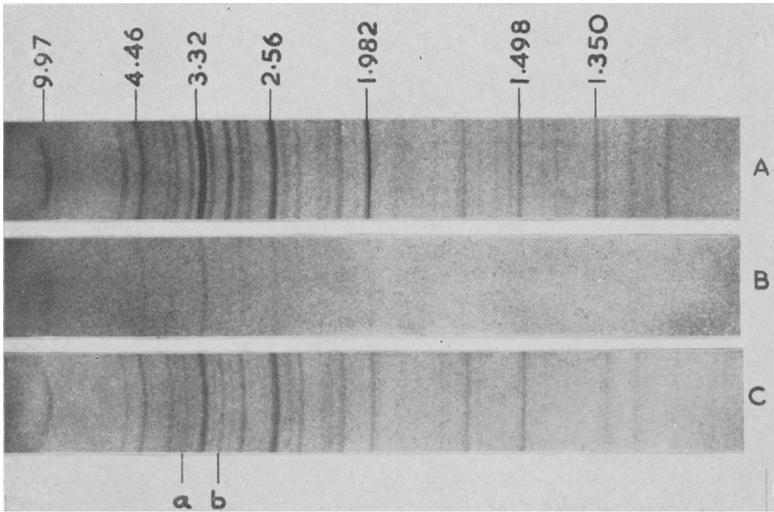
Fig. 2. X-ray diffraction patterns for muscovite samples:
