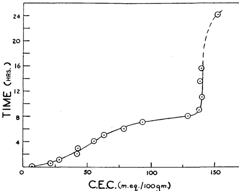
FIG. 1. Relationship between cation-exchange capacity and time of grinding for muscovite.
