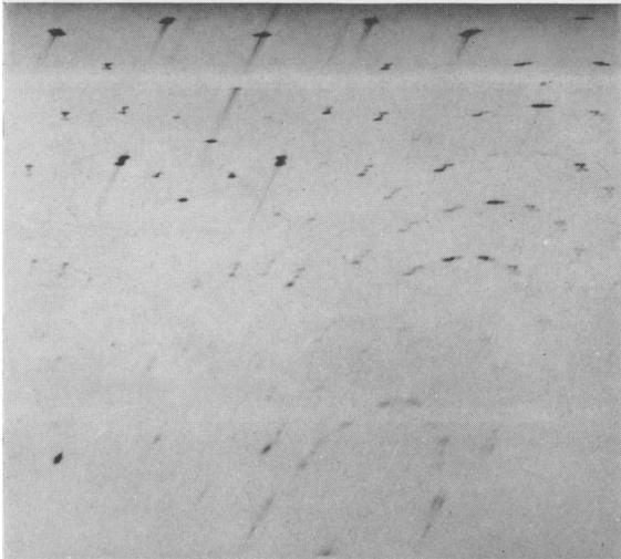
FIG. 3. Zero layer-line Weissenberg photograph taken about the *c*-axis of a fragment of the feldspar from the Bearpaw Mts., Montana, using  $\text{Cu-K}\alpha$  radiation. The reflections from the lattice planes of the five differently oriented units in this crystal are clearly shown and form small crosses in the photograph.
