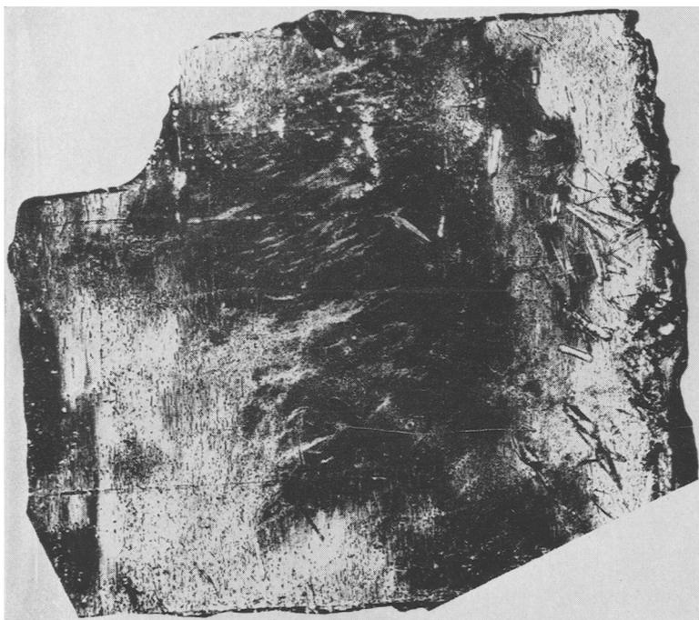
FIG. 2. Photomicrograph of a felspar from a nepheline-syenite pegmatite of Rocky Boy stock, Bearpaw Mts., Montana. The crystal is cut approximately normal to the  $a$  crystallographic axis. The dark areas are monoclinic and the lighter areas are triclinic. Crossed nicols:  $\times 96$ .
