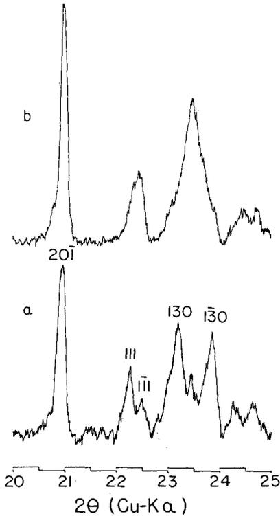
FIG. 5. Parts of the X-ray spectrometer patterns of the feldspars from (a) the Bearpaw Mts., Montana, and (b) Glen Urquhart, Scotland. In pattern (a) the presence of orthoclase is indicated by the reflection between the 130 and  $1\bar{3}0$  reflections of microcline. In pattern (b) the variable lattice of microcline is shown by the broad peaks representing the 130 and  $1\bar{3}0$  reflections and the 111 and  $1\bar{1}\bar{1}$  reflections. By contrast the 201 peak is sharp and well defined.
