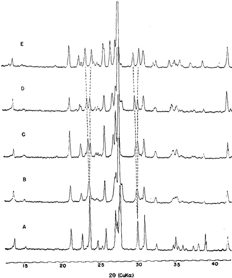
FIG. 1. Powder X-ray diffraction patterns of low-temperature alkali-felspars. Pattern A is of a monoclinic felspar and patterns B, C, D, and E are of microclines with varying departure from monoclinic symmetry. The peak at about  $28^\circ$  ( $\text{Cu-K}\alpha$ ) in patterns B, D, and E is due to the presence of albite as a separate phase.
