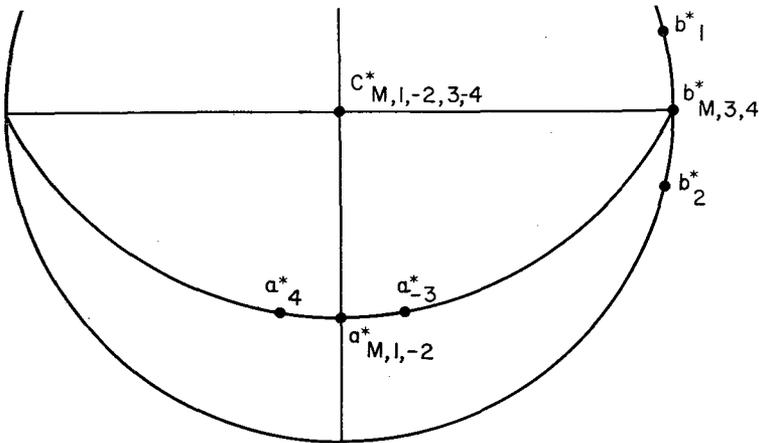
FIG. 4. Stereogram showing the approximate relation between the axes of the reciprocal lattices of the five different units of the felspar from the Bearpaw Mts., Montana. The subscript  $M$  refers to the monoclinic part and the subscripts 1, 2, 3, and 4 refer to the four triclinic parts. The angular relations in the stereogram are very much exaggerated for clarity.
