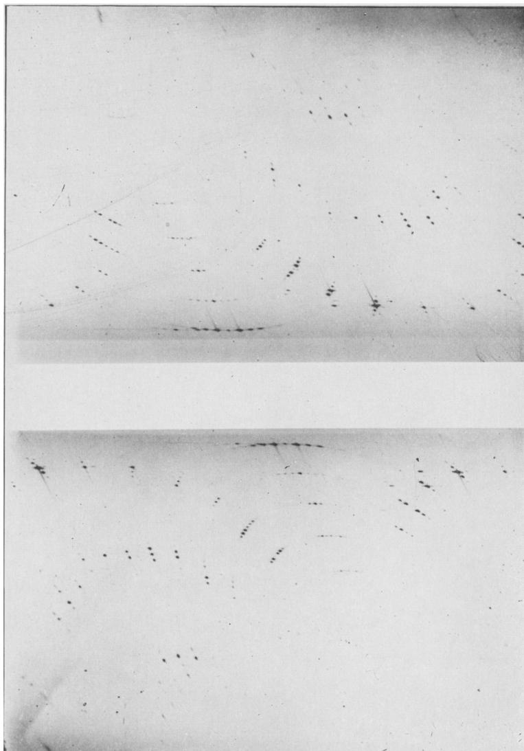
FIG. 2. Antigorite (Mikonnii). Weissenberg ( $h0l$ ) photograph. Ni filtered  $\text{Cu-K}\alpha$  radiation.
