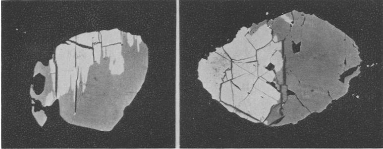
FIGS. 6 and 7: FIG. 6 (*left*). Biotite-diorite, Loch Bad nam Ban. Pyrrhotine (medium grey) and typical 'flame-like' bodies of pentlandite, which prefer basal directions of the pyrrhotine. Reflected light, oil immersion.  $\times 230$ . FIG. 7 (*right*). Biotite-diorite, Loch Bad nam Ban. Pyrrhotine (medium grey), pentlandite (white, excellent cleavage)  $\parallel$  (111), and chalcopyrite (light grey, soft). Reflected light, oil immersion.  $\times 160$ .
