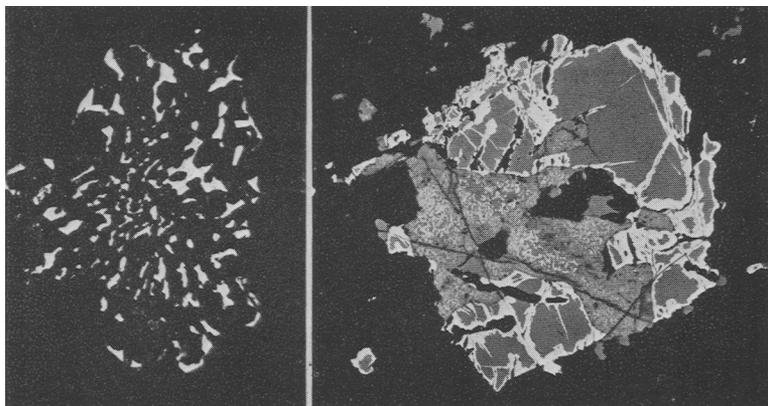
FIGS. 8 and 9: FIG. 8 (*left*). Biotite-diorite, Loch Bad nam Ban. Pyrrhotine (light grey) and pentlandite (white) in graphic intergrowth with silicate mineral. Reflected light, oil immersion.  $\times 160$ . FIG. 9 (*right*). Epidiorite, Allt a Mhuilinn. Magnetite (medium grey) changed into hematite along cracks and grain boundaries; ilmenite has been decomposed to form a fine-grained graphic intergrowth of rutile and hematite. Reflected light, oil immersion.  $\times 160$ .
