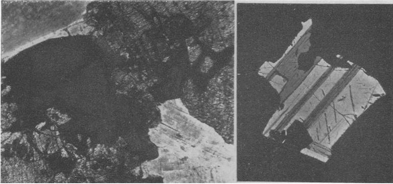
FIGS. 2 and 3: FIG. 2 (*left*). Biotite-diorite, Loch Bad nam Ban. Olivine, augite, biotite, iron ore, plagioclase.  $\times 20$ . FIG. 3 (*right*). Biotite-diorite, Loch Bad nam Ban. Magnetite (light grey) with unmixing lamellae of ilmenite (medium to dark grey, reflection pleochroism)  $\parallel (111)$  and small exsolution bodies of spinel  $\parallel (100)$ . Oil immersion, reflected light.  $\times 250$ .
