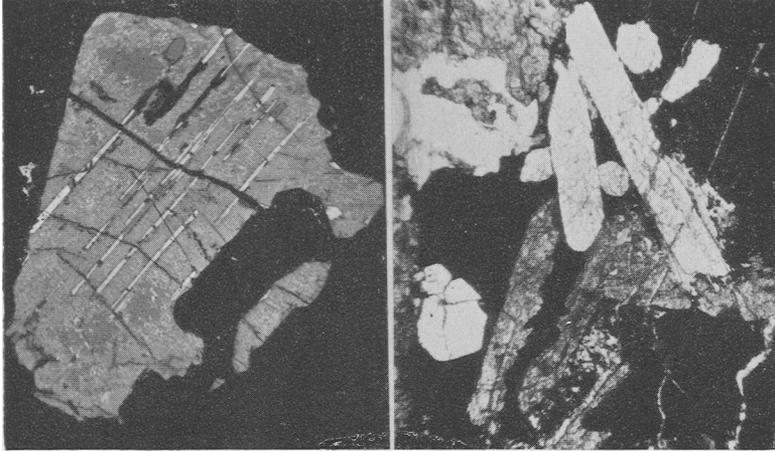
FIGS. 10 and 11: FIG. 10 (*left*). Epidiorite, Allt a Mhuilinn. Ilmenite with (partly oxidized) unmixing lamellae of magnetite  $\parallel$  (0001) ('magnetoilmenite'). The ilmenite is, to a considerable extent, changed into a graphic intergrowth of rutile and hematite. Reflected light, oil immersion.  $\times 160$ . FIG. 11 (*right*). Cromaltite, Bad na h'Achlaise. Typical section, melanite, augite, apatite, magnetite.  $\times 30$ .
