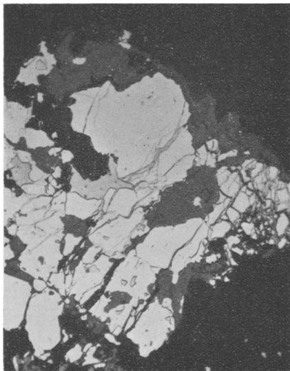
FIG. 12: Cromaltite, Bad na h'Achlaise. Magnetite (dark grey) is replaced by pyrite (white), which in turn is replaced by chalcopyrite (light grey). Reflected light, oil immersion.  $\times 100$ .
