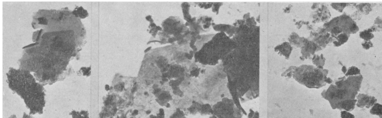
FIG. 1. Electron micrographs showing the close association of delafossite and kaolinite in a specimen from Nizhni Tagil (B.M. 1914, 42); left and centre micrographs, \times 12\ 000 , right \times 9\ 000 .
