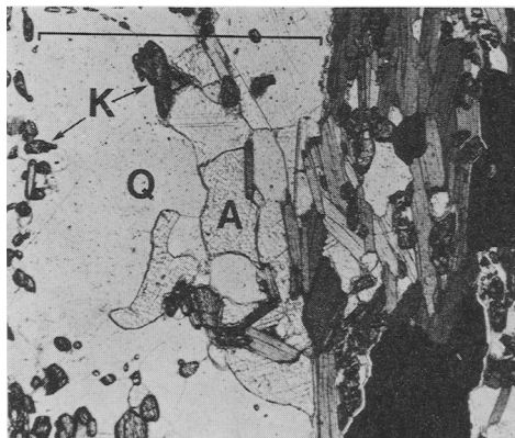
FIG. 1. Photomicrograph of the anhydrite-bearing schist, showing grains of quartz (Q), anhydrite (A), some showing twin lamellae, kyanite (K), and biotite. Note the colourless reaction rims around some of the ore grains. Plane polarized light. Scale bar 1 mm.
