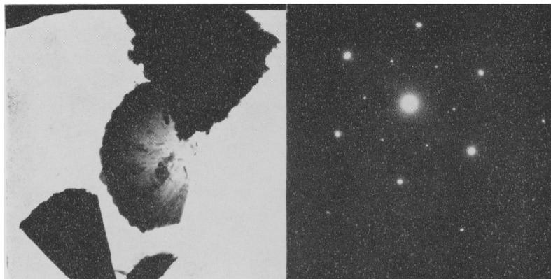
FIGS. 2 and 3: FIG. 2 (left). Electron micrograph of a new phase  $K_2Mn_4O_9$ .
