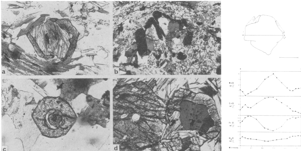
FIGS. 4 and 5: FIG. 4 (left). a. Atoll garnet showing complete replacement of the core by biotite and opaques. Note the preservation of the rims in contact with quartz/feldspar. Specimen C1; plane polarized light; \times 16 diameters. b. Atoll garnet showing replacement of core by biotite, quartz, and a little plagioclase. Mottled texture surrounding the atoll and penetrating the bottom rim is sericite after andalusite. Specimen D15; crossed nicols; \times 16 diameters. c. Atoll garnet showing almost complete isolation of core from the rim by selective replacement of the garnet by quartz and biotite. Specimen C17; plane polarized light; \times 25 diameters. d. Complete and atoll garnets with biotite and some opaques replacing the atoll core. Specimen D15; plane polarized light; \times 16 diameters. FIG. 5 (right). Microprobe traverse across an almost intact thermal garnet from Ar dara. Stippled areas represent biotite and the scale bar is 100 \mu\text{m} . Specimen D12.
