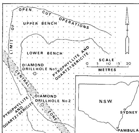
FIG. 1. Plan of the open cut at Back Creek showing locations of the central zone and two of the diamond drillholes.
