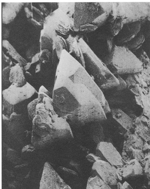
FIG. 1. Scanning electron micrograph ( \times 70 ) showing a pseudotrigonal contact triplet.
