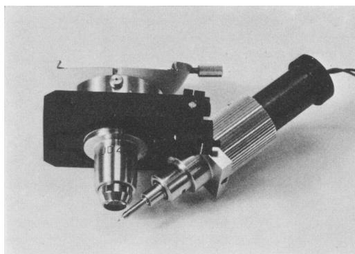
FIG. 1. Micro-drill mounted on a centrable holder for single objectives. A drill rod furnished with a polished monocrystalline diamond tip is in the pin-vice of the drill.
