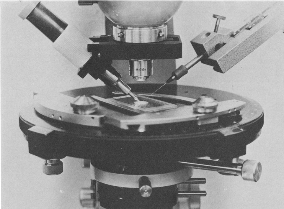
FIG. 2. Detail of the micro-drill during a drilling operation. Rotary stage with mechanical stage holding a polished thin section, objective holder with micro-drill, micromanipulator holding metal tube with rubber mouthpiece. In the mouthpiece the hollow cylindrical X-ray camera mounting plinth with microcapillary can be seen.
