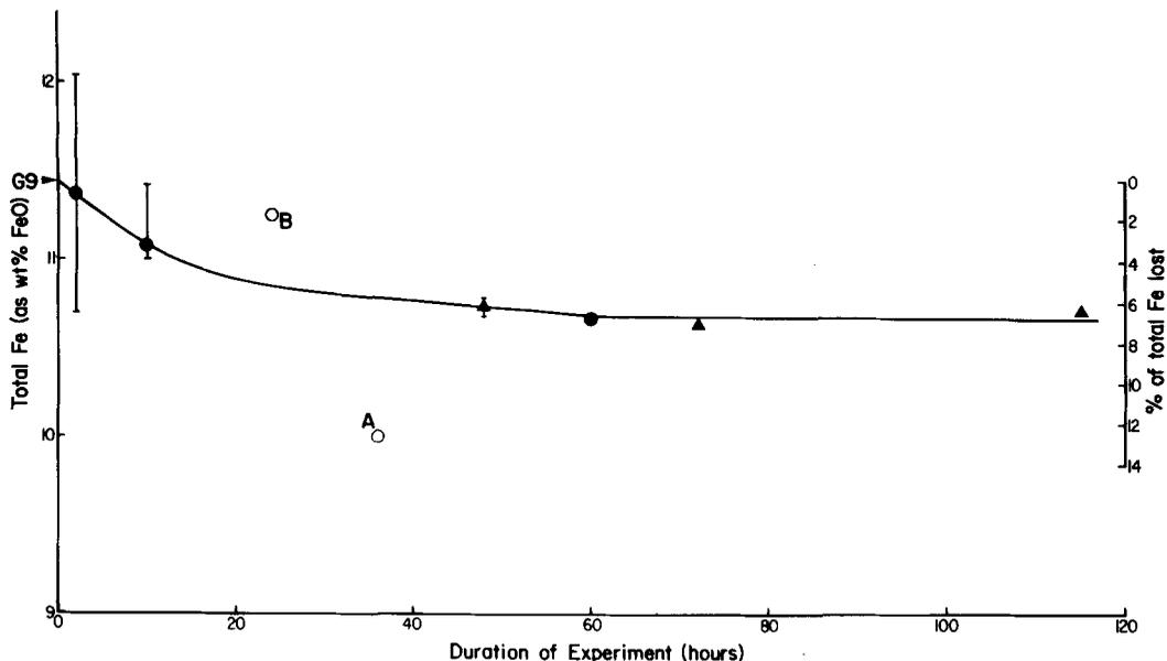
FIG. 1. Average Fe contents of quenched glasses from experiments on basalt G.9 using 0.2-mm-diameter  $\text{Ag}_{40}\text{Pd}_{60}$  wire loops. Vertical bars indicate the range of Fe contents determined by electron-probe spot analyses. The symbols are explained in the text.
