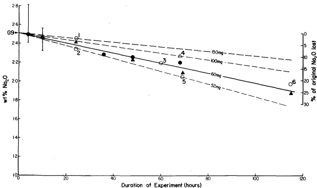
FIG. 2. Average Na<sub>2</sub>O contents of quenched G.9 glasses from experiments using loops of Pt (▲) and Ag<sub>40</sub>Pd<sub>60</sub> (●) wire. Solid symbols represent samples with an initial weight between 55 and 65 mg. Numbered open symbols represent lighter or heavier samples (see Table II). Vertical bars give the range of individual spot analyses.
