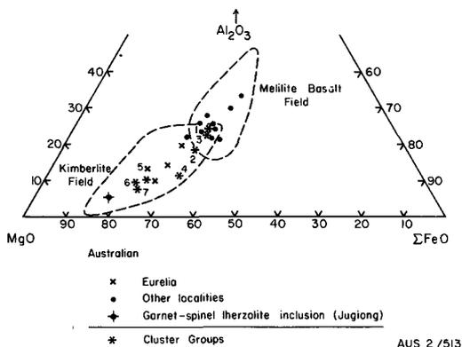
FIG. 2.  $Al_2O_3$ -MgO-total FeO diagram for kimberlitic rocks of southeastern Australia, showing kimberlite and melilite basalt fields of Cornelissen and Verwoerd (1975). Also indicated are the compositions of a garnet-spinel lherzolite nodule from Jugiong, the kimberlitic cluster groups (1–7) of McIver and Ferguson (1979).
