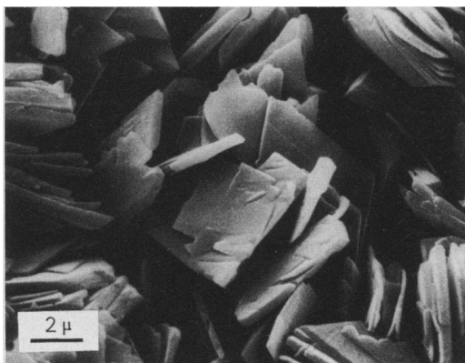
FIG. 2. Scanning electron micrograph of basaluminite from Chickerell.
