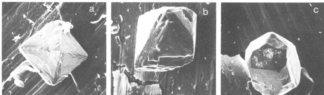
FIG. 1. SEM micrographs, field of view approximately 0.3 mm. (a) gahnite showing octahedral form, (b) gahnite displaying both octahedral and dodecahedral forms, (c) columbite.
