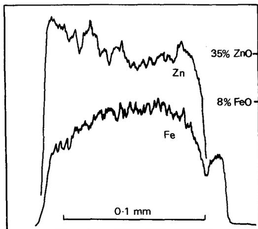
FIG. 2. Zn and Fe zoning in gahnite (microprobe scan). The FeO peak at approximately 4% on the right-hand side represents adjoining muscovite
