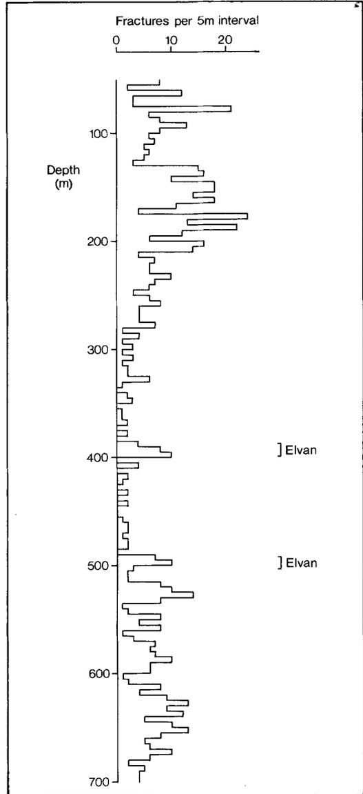
FIG. 4. Fracture frequency, Borehole 8.
