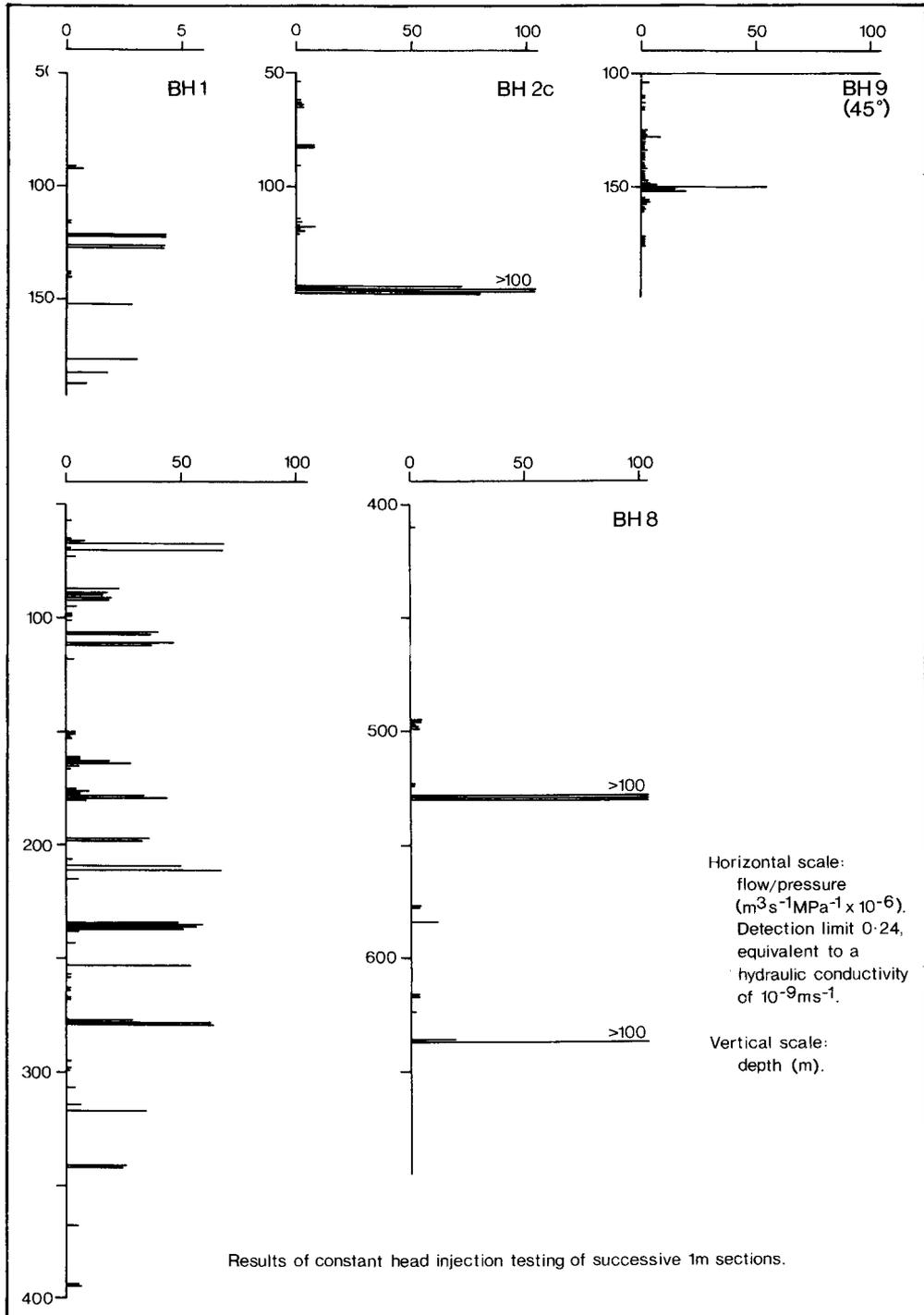
FIG. 3. Results of hydraulic tests, Troon test site.
