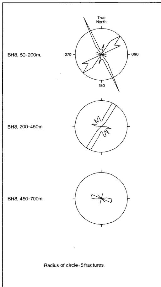
FIG. 6. Orientation of water-conducting fractures, Troon test site.
