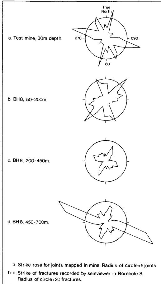
FIG. 5. Fracture orientation, Troon test site.
