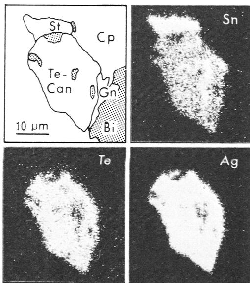
FIG. 2. Sketch and X-ray image for Sn-L $\alpha$ , Te-L $\alpha$ , Ag-L $\alpha$ , showing the element distribution of a typical assemblage with Te-bearing canfieldite (Te-Can), stannite (St), galena (Gn), bismuth (Bi), and chalcopyrite (Cp). Specimen 4W4, Panasqueira.
