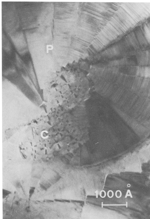
FIG. 5. Almost complete polygonal serpentine fibre (p), with chrysotile (c) core.
