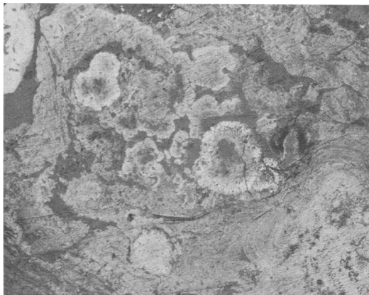
FIG. 1. Optical micrograph of polished section of Groote Eylandt manganese ore showing co-existing todorokite (white) and vernadite (grey). \times 280 .
