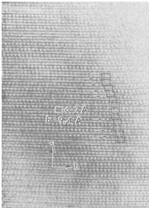
FIG. 8. High resolution electron micrograph showing  $b/3$  layer stacking faults in chamosite (from Barber, 1985; micrography by J. Akai).
