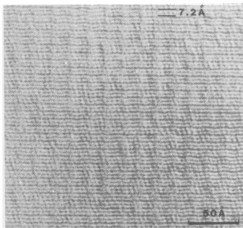
FIGS. 6 and 7. FIG. 6 (left). Idealized version of the tetrahedral component of the structure of greenalite or caryopilite. FIG. 7 (right). High-resolution electron micrograph of caryopilite showing corrugated layer structure (both from Guggenheim *et al.*, 1982).
