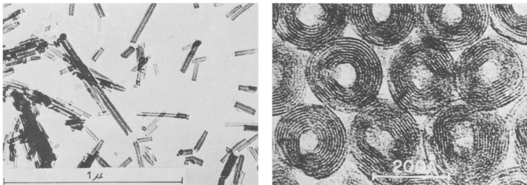
FIGS. 1 and 2. FIG. 1 (left). Electron micrograph of synthetic chrysotile (from Whittaker and Zussman, 1971). FIG. 2 (right). High-resolution electron micrograph of cross-section of chrysotile asbestos (Yada, 1971).
