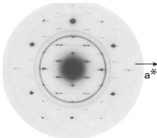
FIG. 3. Electron diffraction pattern of antigorite (Glen Urquhart, Scotland) with  $a$  35 Å. Closely spaced lines of spots in the  $a^*$  direction are in clusters relating to the simple cell with  $a$  5.3 Å,  $b$  9.2 Å. Powder rings are from Pt coating.
