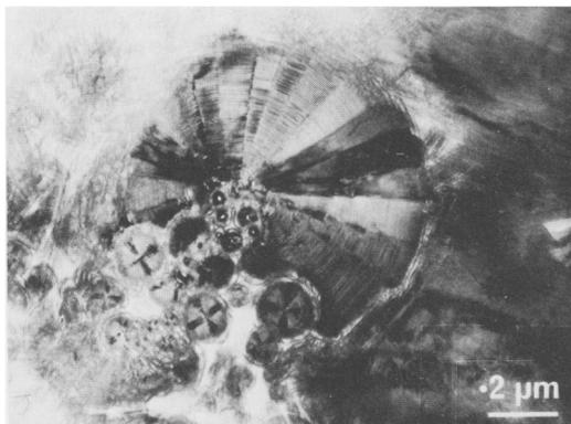
FIG. 5. Electron micrograph of polygonal chrysotile (Cressey and Zussman, 1976).
