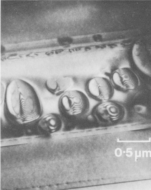
FIG. 13. Electron micrograph of ion-thinned 'byssolite' crystal showing what are probably fluid inclusions or voids.
