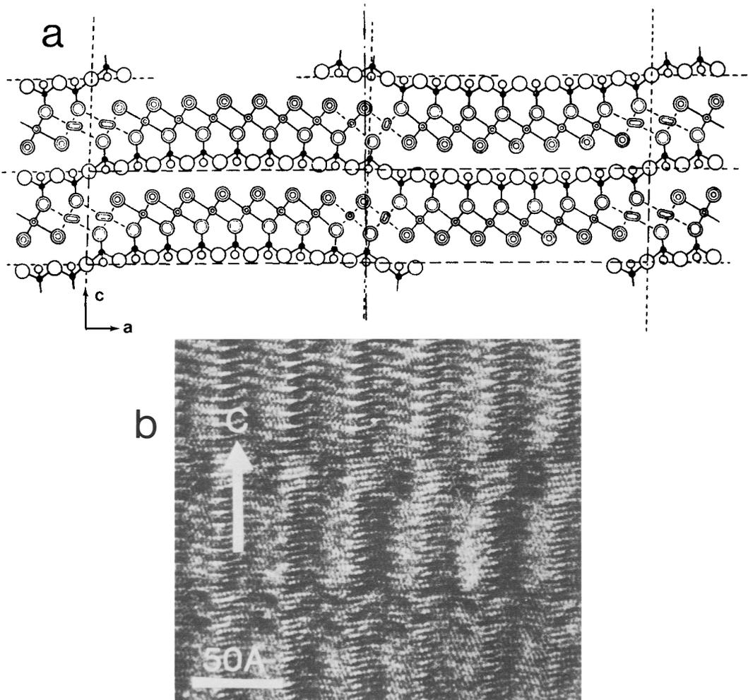
FIG. 4. (a) Corrugated layer structure of antigorite as viewed along the  $y$  axis (X-ray determination; Kunze, 1956). (b) High-resolution electron micrograph of antigorite; electron beam parallel to  $y$  axis (Cressey and Hutchison, 1983).
