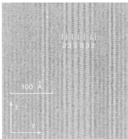
FIG. 12. High-resolution electron micrograph of Zn-tremolite asbestos showing an ordered region of triple chain structure (Dorling and Zussman, 1984).
