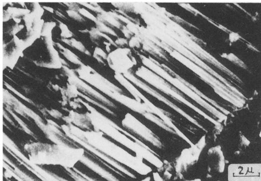
FIG. 1. Scanning electron micrograph showing fibrous crystals of merlinoite in a manganese nodule cavity.
