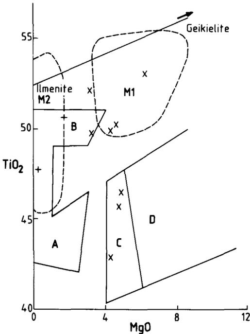
FIG. 4. Plot of MgO vs. TiO<sub>2</sub> in ilmenite. Crosses represent Lebombo picrites; pluses Lebombo low-MgO basalts. Fields M1 and M2 from Mount Ayliff are explained in Fig. 3. Note the high TiO<sub>2</sub> content of MgO-rich ilmenites from both localities. Typical fields of ilmenite compositions are from Haggerty (1976). A, ilmenites from felsic rocks; B, tholeiitic rocks; C, alkali basaltic rocks; D, kimberlites.
