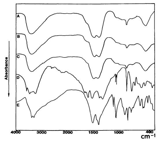
FIG. 1. Infrared spectra of: A, georgeite, Carr Boyd Mine (original sample in KBr disc used for infrared study by Bridge *et al.*, 1979); B, georgeite, Britannia Mine; C, synthetic georgeite, Cu<sub>2</sub>CO<sub>3</sub>(OH)<sub>2</sub>; D, chalconatronite; E, malachite. The latter two samples are synthetic materials confirmed by X-ray powder diffraction methods.
