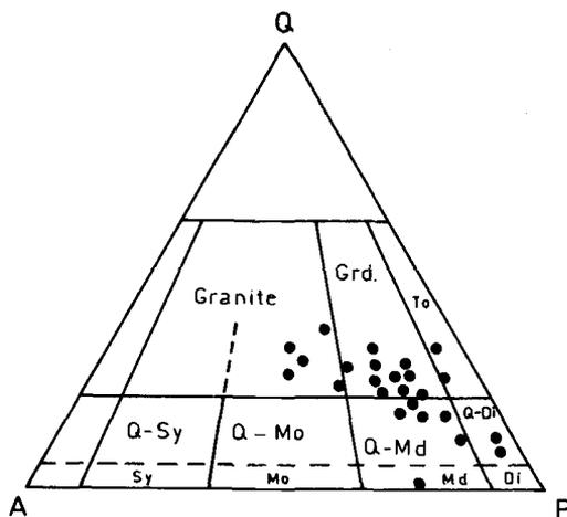
FIG. 3. Modal analyses of 25 samples plotted on the classification diagram recommended by Streckeisen (1976).
