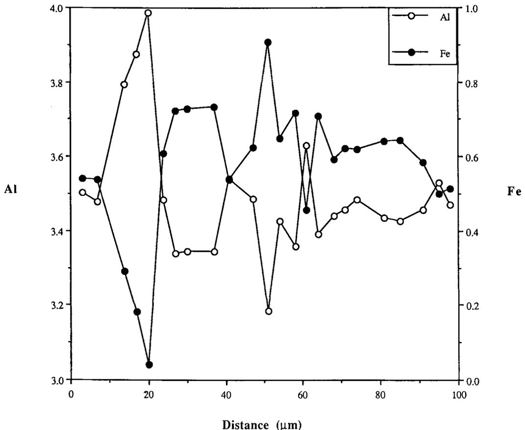
FIG. 2. Microprobe traverse along the line A (left) to B (right) shown on Fig. 1. Analyses are expressed as nos. of atoms per formula unit.
