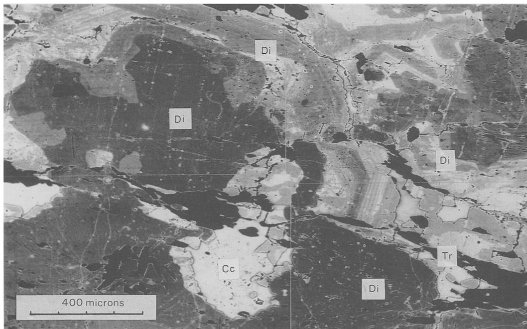
FIG. 4. Mosaic of BSEM photomicrographs of diopside rock from Connemara, Ireland. Diopside grains (Di) have homogeneous cores of dark (Mg-rich) diopside, cut by veinlets of lighter, more Fe-rich diopside. The cores have corroded outlines but are overgrown by oscillatory zoned diopside which develops a euhedral shape. Black grains, often lozenge shaped, are tremolite (Tr), white grains and crack fills are of calcite (Cc).
