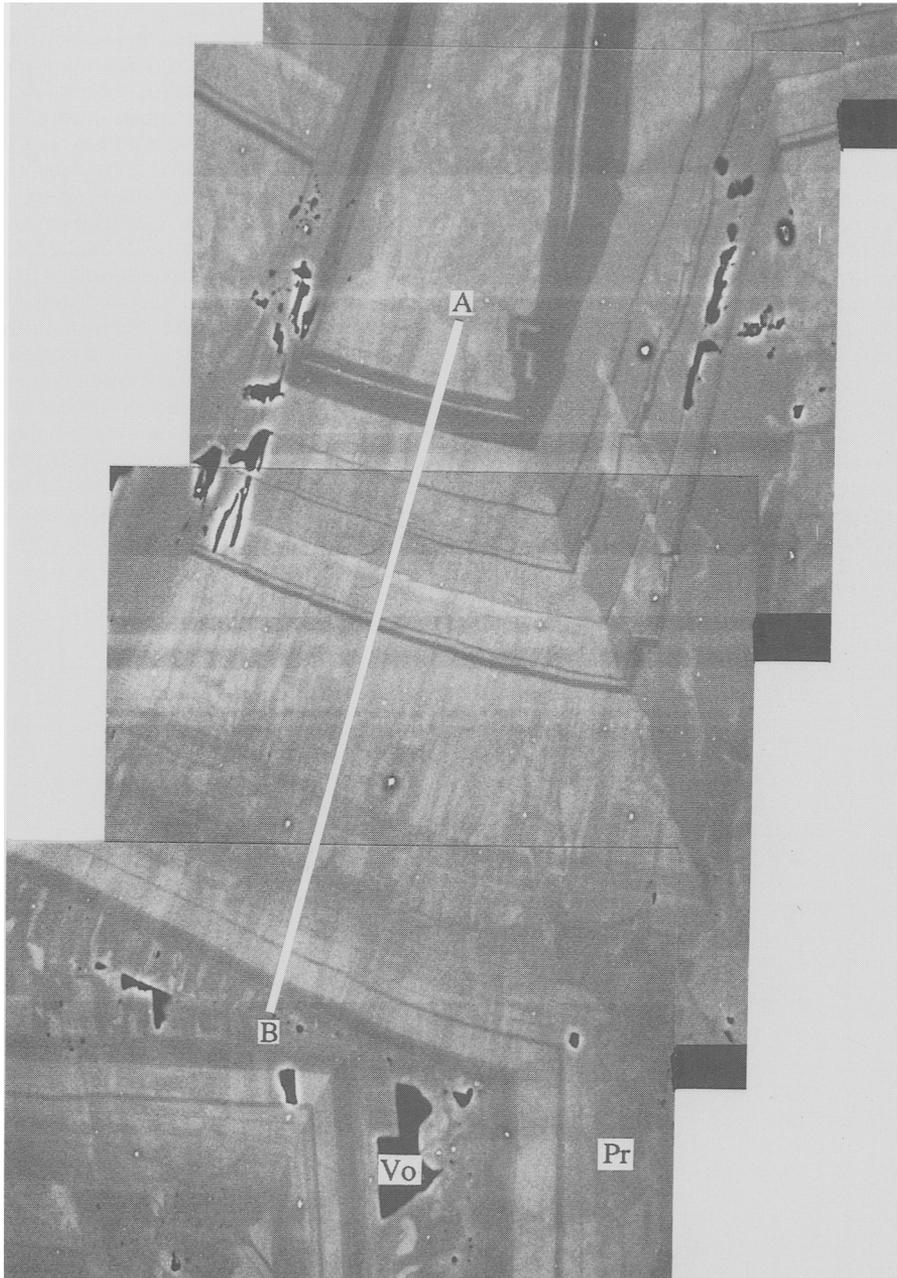
FIG. 1. Back Scattered Electron Microscope (BSEM) image of zoned prehnite (Pr), occurring in a vein at *c.* 970 m depth in well PGM11, Mirvalles geothermal field, Costa Rica. Vo denotes a void. Light bands are of higher mean atomic number (i.e. contain more Fe). A microprobe traverse along the line A–B is shown in Fig. 2.
