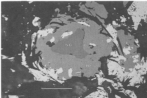
FIG. 6. Anhedronal ferritchromite grain from Salamanca district associated with serpentine minerals and sulfides, where it is possible to distinguish the core (Sc), which in its lower left corner show a narrow darker zone (with higher  $\text{Al}_2\text{O}_3$  content) and in its upper left corner a very small silicate inclusion in contact with the outer B rim; the B rim (Br) shows sulfide and silicate inclusions. Scale bar represents 60  $\mu\text{m}$ .
