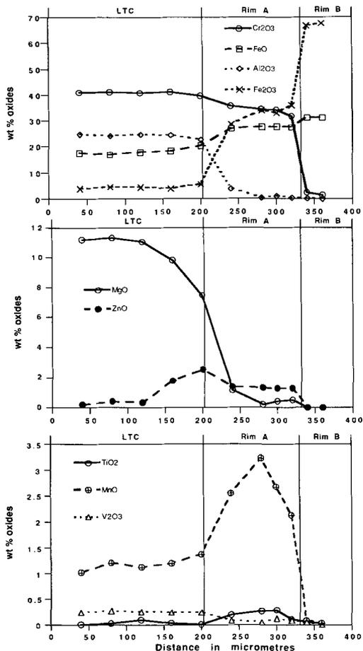
FIG. 4. Compositional variations from the centre of the core to rim B in one chromite grain from Las Tunas area.
