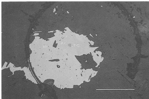
FIG. 5. Anhedronal chromite grain from Las Tunas area, in a silicate matrix, which shows a small (LTC) core surrounded by a wide A rim (Ar) which outwards is succeeded by a B rim (Br). Scale bar represents 160  $\mu\text{m}$ .
