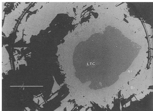
FIG. 3. Chromite grain from Las Tunas area included in serpentine matrix, with well developed zonation: (LTC) the core, (Ar) the A rim and (Br) the B rim; silicate inclusions restricted to the contact between the latter two. Scale bar represents 125  $\mu\text{m}$ .
