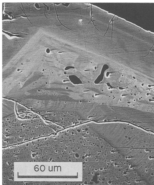
FIG. 3. Back scattered electron image showing resorption pores, complex zoning and domain structures in the inner mantle of a tausonite crystal.
