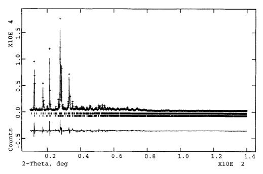
FIG. 1. Observed, calculated and difference profiles for the Magheramorne gobbinsite. Lower Bragg peak marks are for gobbinsite, upper marks are for phillipsite.
