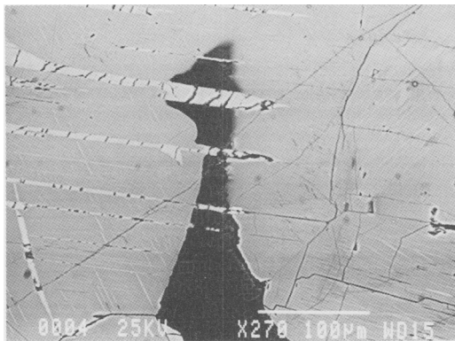
FIG. 4. Electron backscatter image of low-Ca pyroxene lamellae, exsolved from augite, extending into and across areas of intercumulus plagioclase (sample 420, cycle III). Plagioclase is black, augite mid-grey, and low-Ca pyroxene pale grey.
