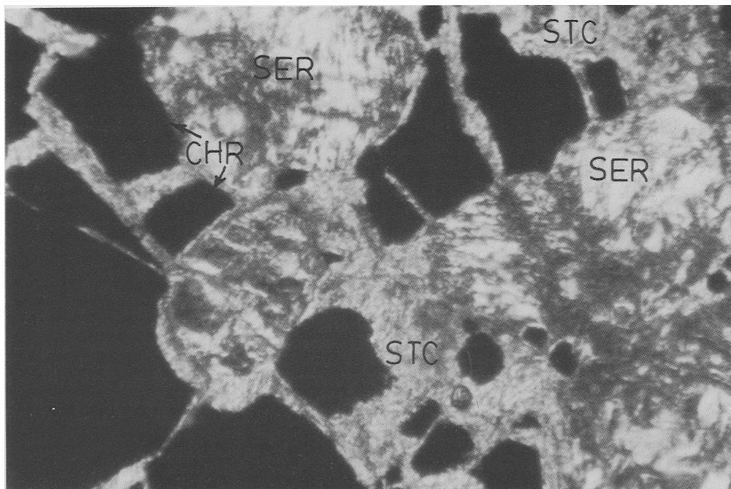
FIG. 1. Photomicrograph showing fracture-filling stichtite in association with chromite and serpentine. Under crossed polars. Length of the figure is 1.6 mm. (STC = Stichtite, CHR = Chromite and SER = Serpentine).
