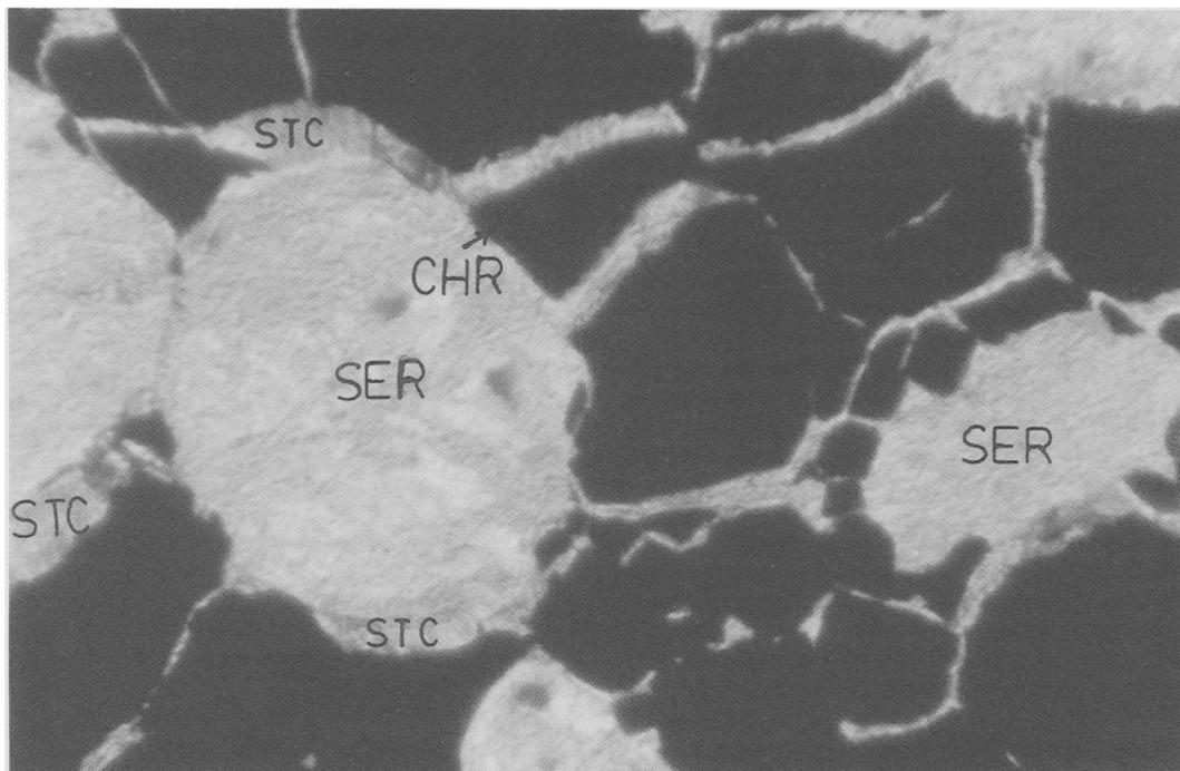
FIG. 2. Photomicrograph showing interstitial stichtite in association with serpentine and chromite. Under plane polarised light. Length of the figure is 1.6 mm. (STC = Stichtite, CHR = Chromite and SER = Serpentine).
