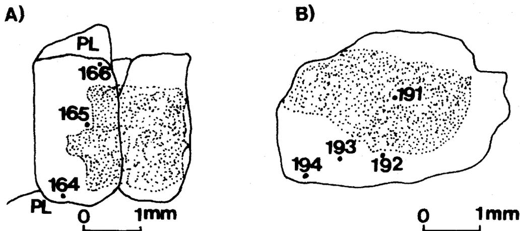
FIG 9. Electron microprobe analyses locations for two sericitized plagioclase grains. The numbers shown are the serial numbers of probe analyses.
