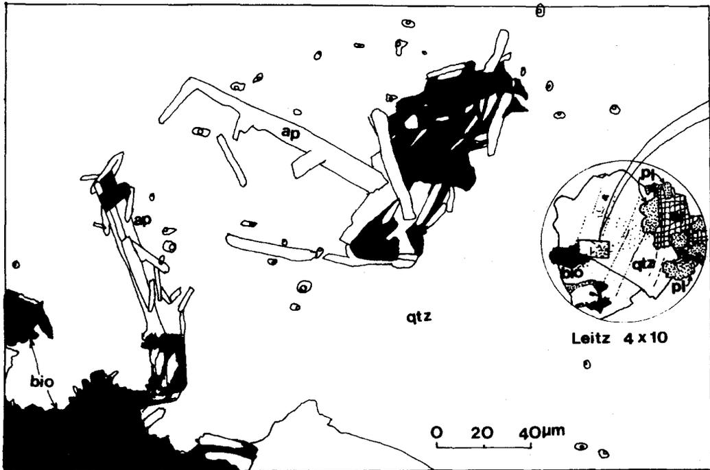
FIG. 10. Biphase fluid inclusions in quartz together with apatite crystals forming as a biproduct of the chloritization of biotite. Inset shows the relationships of the host quartz in the thin section. af = alkali feldspar, ap = apatite, bio = chloritized biotite, pl = plagioclase, qtz = quartz.
