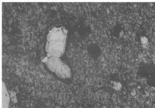
FIG. 8. Phenocrysts of calcite in phonolite N 2003, under crossed nicols. Magnification \times 100 .
