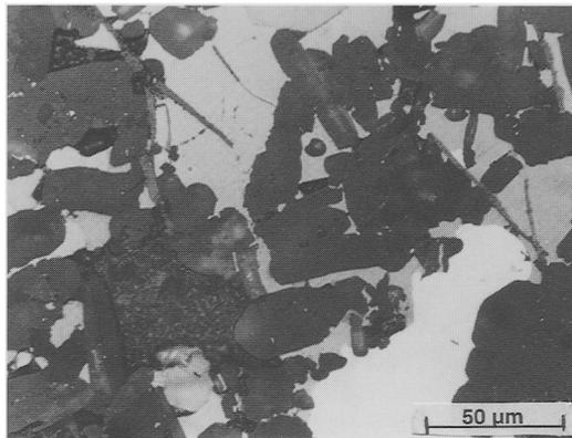
FIG. 1. Reflected light photomicrograph of branching euhedral graphite laths (medium grey, upper left and far right) in the Abee EH enstatite chondrite. The graphite laths occur inside troilite (light grey) and adjacent to silicate grains (dark grey). White region at bottom right is kamacite. The graphite laths, which closely resemble primary igneous graphite in terrestrial ultramafic rocks, most likely crystallized from an enstatite-chondrite impact melt.
