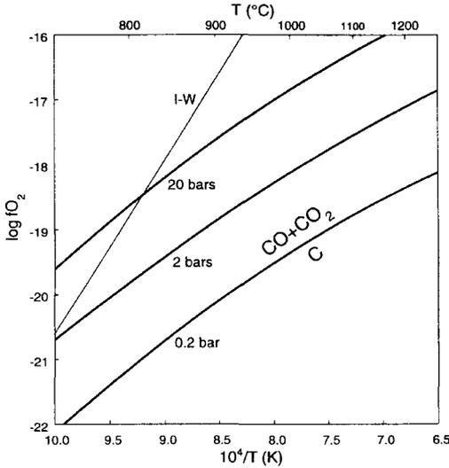
FIG. 2. Variation in the  $\log f_{\text{O}_2}$  values of the graphite surface (i.e. the C-CO+CO<sub>2</sub> buffer) with temperature. There is a positive correlation between  $\log f_{\text{O}_2}$  and pressure. The iron-wüstite (I-W) buffer is shown for reference. After Brett and Sato (1984).
