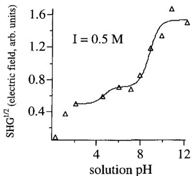
FIG. 1. pH-dependent SHG signal from the silica-solution interface as a function of pH. The two-pK model fit gives estimates of 4.6 and 8.8 for the two surface silanol pKs.
