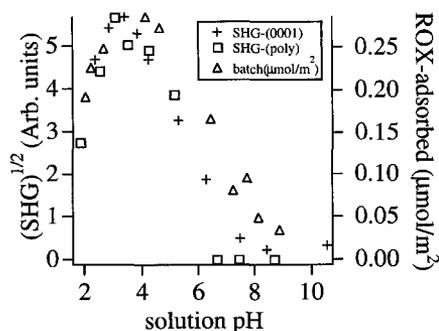
FIG. 3. SHG signal for 5,6-ROX adsorption as a function of pH, compared to stoichiometric experimental batch results. A maximum adsorption occurs at about pH 3.5, in rough agreement with surface complexation models for other dicarboxylic acids (Kummert and Stumm, 1980; Kallay and Matijevic, 1985).
