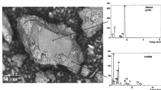
FIG. 2. SEM micrograph of a silicate grain and corresponding EDS spectra.
