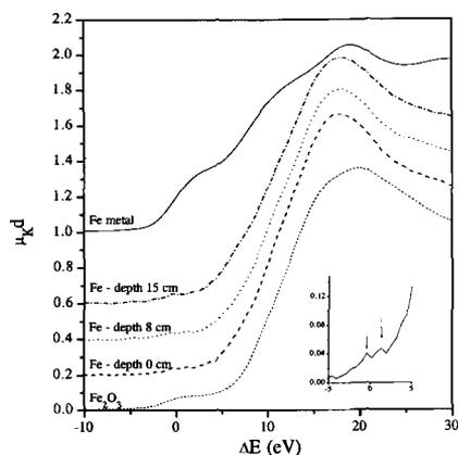
FIG. 3. Normalized Fe K-edge profiles, displaced vertically, for the sediment and reference samples. Energy scale is relative to the Fe K-edge in Fe metal (7112 eV). The average of the three spectra measured in sediment in the energy region of the pre-edge resonances (indicated by arrows) is shown in the inset.
