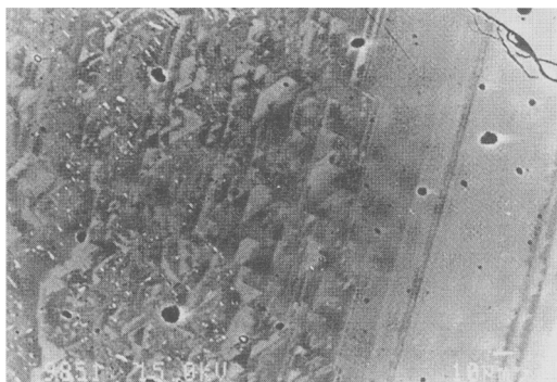
FIG. 2. Back Scatter Electron image of a pyrite sample. Light grey areas correlate with relatively As-rich zones within the sample, dark areas correspond to As-poor zones.
