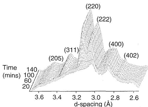
FIG. 2. Time resolved EDPD trace showing the formation of tobermorite at 270°C.
