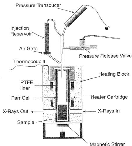
FIG. 1. Schematic diagram showing on-line hydrothermal synthesis equipment.
