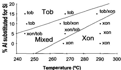
FIG. 3. Summary of all hydrothermal synthesis runs showing the zones where tobermorite and xonotlite formed as a function of temperature and Al content.
