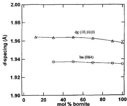
FIG. 5. Variation in  $d$ -spacing with bulk composition for coexisting bornite and digenite  $\{220\}$  peaks at room- $T$ , indexed to the relevant low supercells. Digenite data at 100 mol.%  $bn$  refers to position of trace digenite peak seen in Magma Mine bornite sample in Fig. 3.  $Bn_{90}$  sample has been quenched from 450°C and all other samples were quenched from 600°C.
