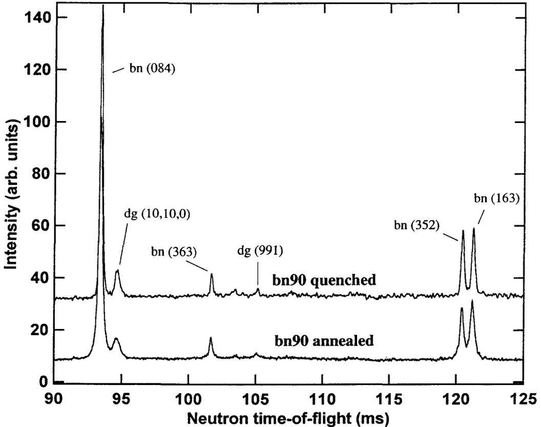
FIG. 7. Expanded section of the 85–165 ms TOF window for  $bn_{90}$  sample quenched from 450°C, and annealed at 180°C for 11 weeks. In the annealed sample the peak broadening is given by FWHM values of  $295.5 \pm 2.0$  ms and  $517.3 \pm 21.0$  ms for the bornite (084) and digenite (10,10,0) peaks respectively. For the quenched sample the equivalent values are  $159.7 \pm 1.7$  ms and  $355.1 \pm 14.5$  ms.
