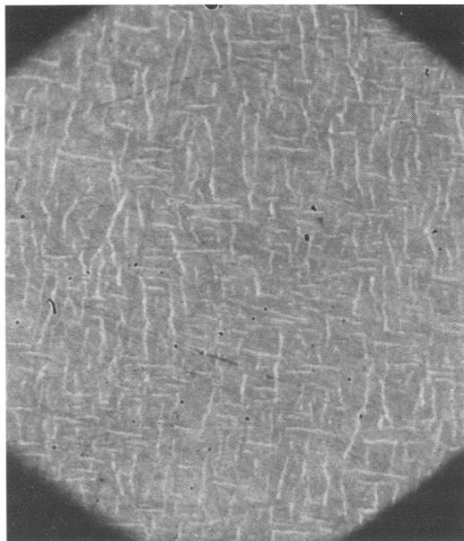
FIG. 2. Photomicrograph of the annealed sample of composition  $bn_{90}$  taken in reflected light, showing the characteristic 'basket-weave' microstructure defined by digenite lamellae. Observed proportions of bornite and digenite mirror the bulk composition. Field of view is 75  $\mu\text{m}$ .
