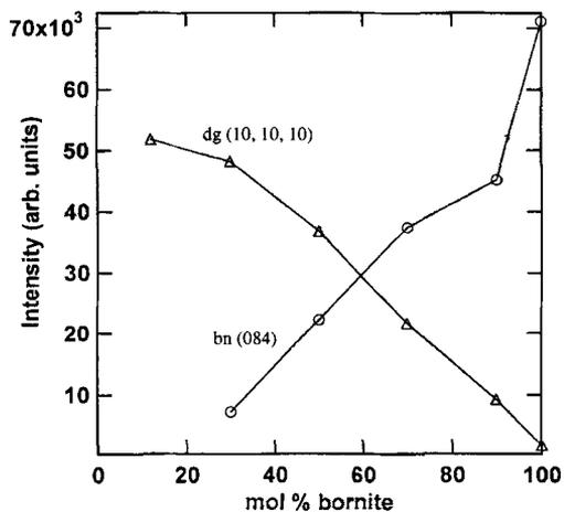
FIG. 6. Intensity variation of bornite and digenite Bragg peaks across the solid solution. Data collected from quenched samples at room- $T$ .
