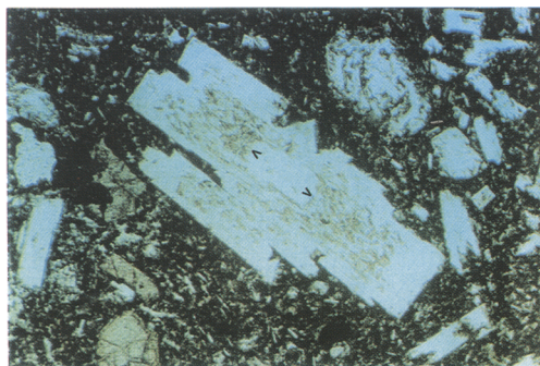
PLATE 8. PPL photomicrograph of a plagioclase phenocryst from the water quenched 1983 lava of Etna (sample DK5) showing a concentric zone of glass inclusions, indicated by tick marks.
